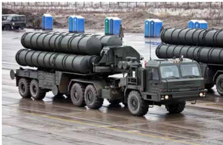
S-400 Triumph air defence system transporter erector launcher. Photo by Vitaliy Kuzmin, available for use under the Creative Commons Attribution-Share Alike 4.0 International licence.
