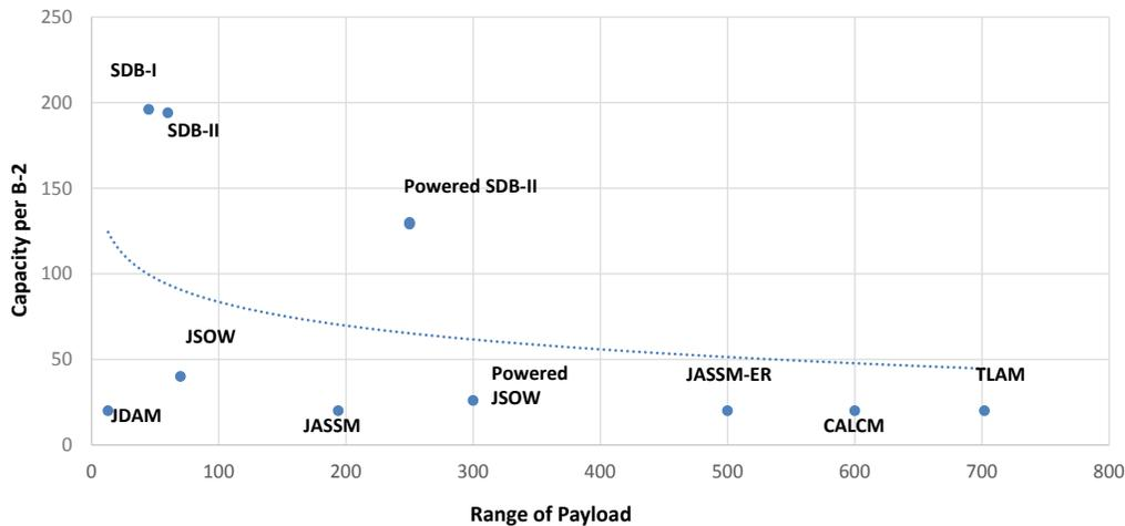
42 The figure uses a total payload capacity of 40,000 lbs. for the B-2, and the weights of each weapon type. For powered glide bombs that do not have propulsion systems, the propulsion system is expected to weigh 50 percent of the weight of the weapon, which was considered a conservative estimate that addresses the potential impact of the propulsion system on the weapon's form factor and ability to fit in the B-2 payload bay.
