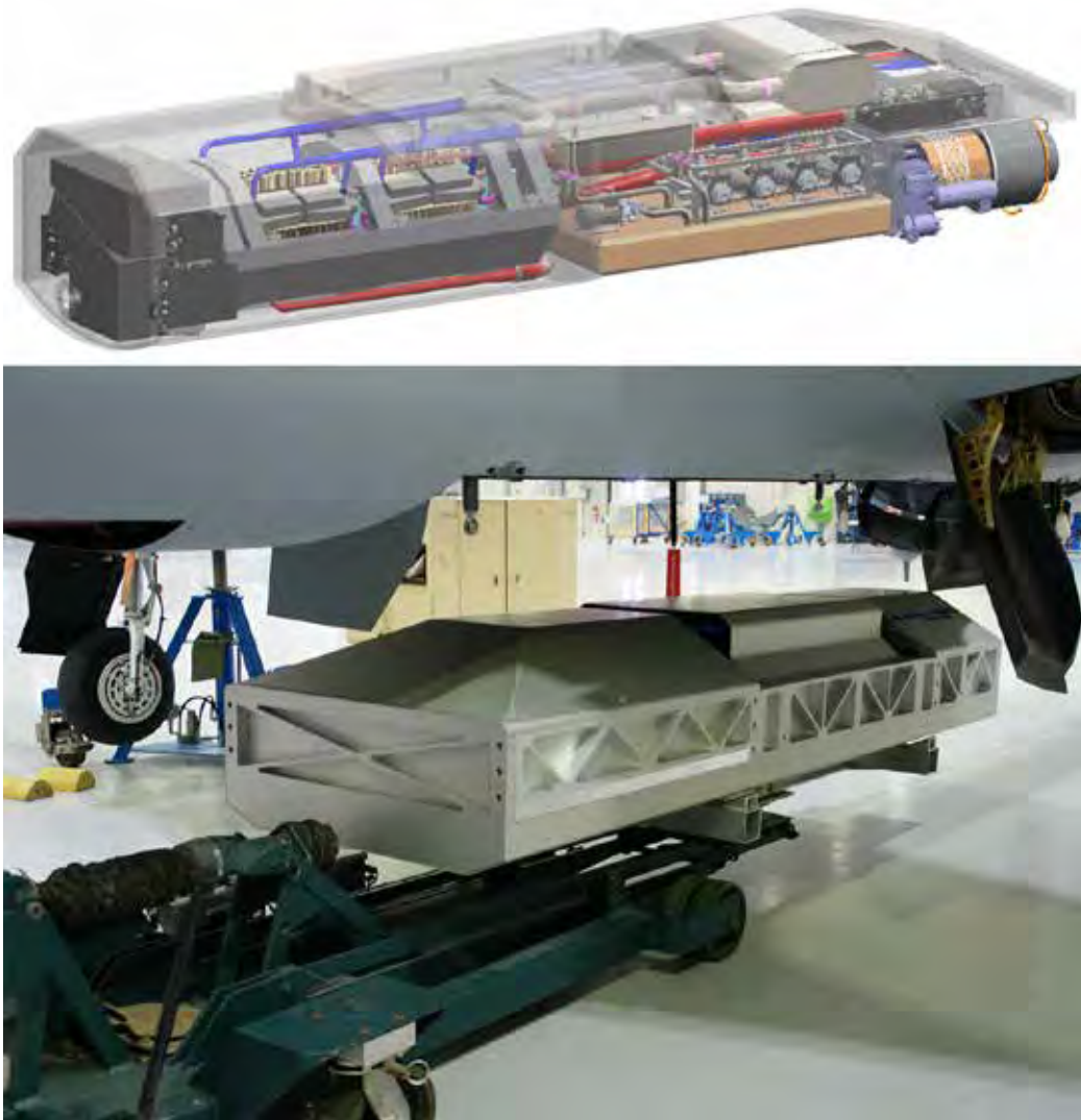
FIGURE 13: DEVELOPMENTAL 100 KW-CLASS LASER CONFIGURED TO INTEGRATE WITH A UAV
