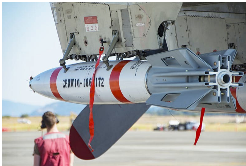
FIGURE 7: QUICKSTRIKE ER WITH TAILFINS TO EXTEND ITS RANGE
